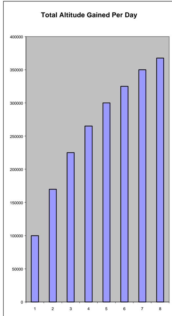
The graphic above calculates the productivity, (defined as total height gained, launches and revenue per day), resulting for the use of a multi-drum winch with 1 – 8 drums. The starting assumptions are in the box in the upper left. The two minute launch interval has been confirmed by the *Amsterdam Soaring Club*.
