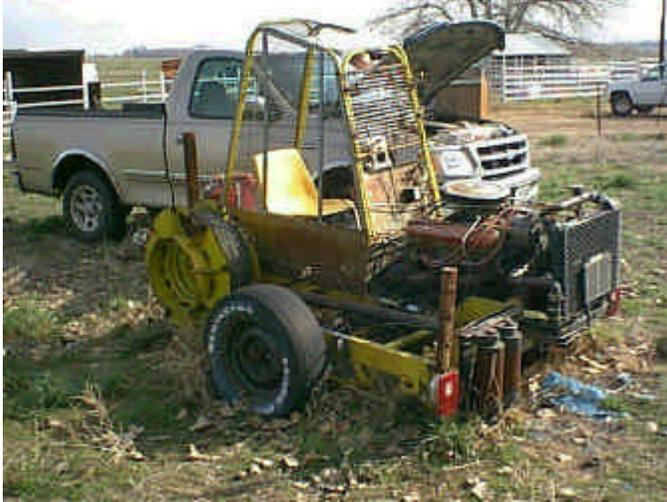
Typically, glider winches in the US are scratch built by volunteer members of glider clubs. They almost invariably use auto/truck V8 engines and automatic transmissions driving one drum through a locked differential in a solid axle. These parts are almost always obtained from wrecked cars in junkyards.
