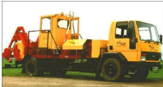
The SupaCat winch uses a level-wind, paying-on mechanism and large swiveling pulleys.
