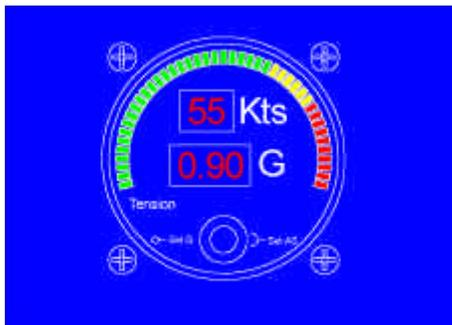
The pilot would set the desired airspeed and initial acceleration on a panel instrument which, in turn, would send these data to the winch by a radio telemetry link. Once the launch is underway, this link would send real-time acceleration, airspeed and altitude data to the winch.
