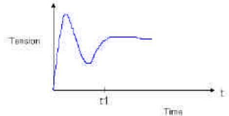
Tension should be monitored at the glider with the information presented to the pilot since the pilot is in the best position to control tension with back pressure. Tension load cells equipped with short distance “Bluetooth” wireless links are inexpensive and small enough to be inserted into the winch cable at the parachute. The safe tension values would be color marked on the glider panel instrument.
