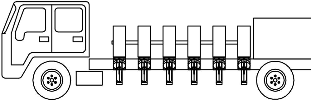
**Possible 6-Drum "Sidewinder" Truck Mounted Winch with Separate Winch Engine**
