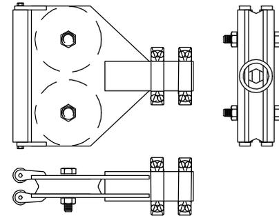
**Tost Style Azimuth Rollers**
