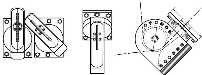
**Inclined Swivel Pulley**
